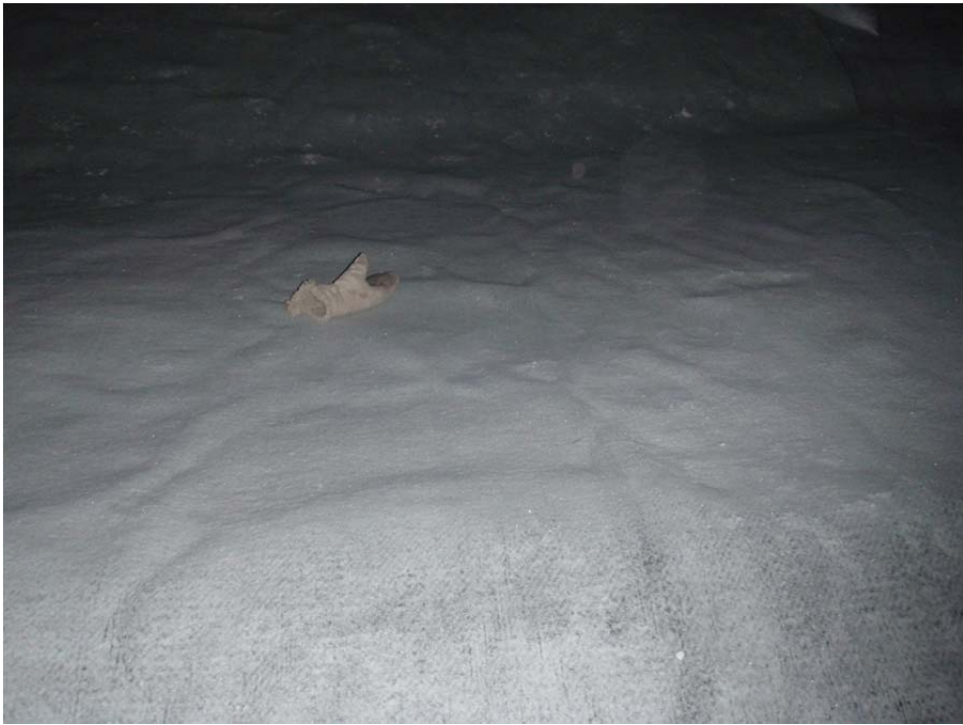
Photo 12 (left): View of some minor wrinkles observed in the stiff (partially frozen) GCL.
